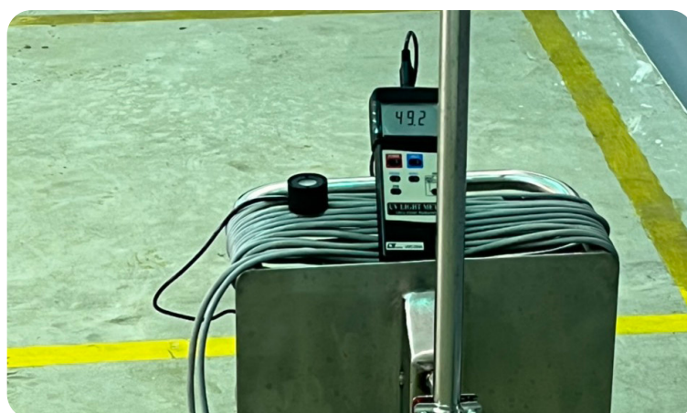
UVC Radiometer testing the UVC Intensity
