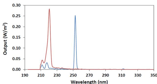
Figure 3. Spectral discharge ( $\text{W m}^{-2}$ ) from a 55-W UV-C (254 nm, low-pressure mercury lamp (blue line) and 250 W 222 nm Krypton Chloride excimer lamp (red line) measured with a fiber optics StellarNet spectrometer at 30-cm distance from the lamp. The 254 nm mercury lamp also emitted 3% of its total irradiance in 210 to 215 nm range.
