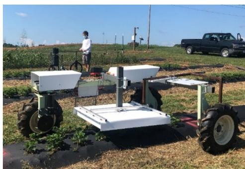
Figure 1. A second-generation autonomous UV-C application platform undergoing trials at the Appalachian Fruit Research Station, in Kearneysville, WV in a research plot established to study the infestation of strawberry plants by pestiferous arthropods. The robot has a computer vision system to simultaneously capture images for later analysis. The person in the background is manually capturing images of strawberry plants with a camera mounted on a pushcart.
